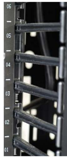
Vertical cable managers maintain organized cables at each u space and simplify cable routing and installation. 6 inch depth cable fingers can accommodate 50+ cat6 cables
